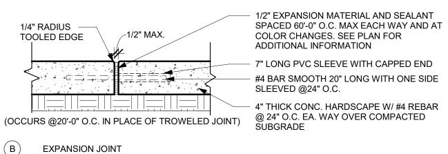
1/4" RADIUS TOOLED JOINT 3/16" WIDE BY 1/2" DEEP SPACED 5'-0" O.C. MAX. EACH WAY PER PLAN - 4" THICK CONC. HARDSCAPE W/ #4 REBAR @ 24" O.C. EA. WAY OVER COMPACTED SUBGRADE NOTE: CONCRETE SHALL BE AT LEAST AS SLIP RESISTANT AS A MEDIUM BROOM FINISH
